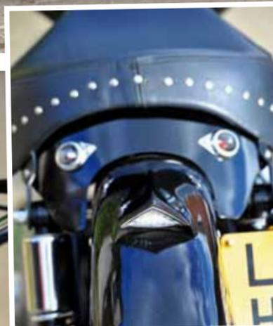
model) front mudguard. The fuel tank is a modified long-range one that's had its bottom cut out and a box welded into it to take the electrics and keep the space under the seat just that... a space. And the seat is equally as clever - it's a one-off with a fabricated panel below that holds the rear indicators unobtrusively. The indicators, front and rear, are modified Royal Enfield side-
